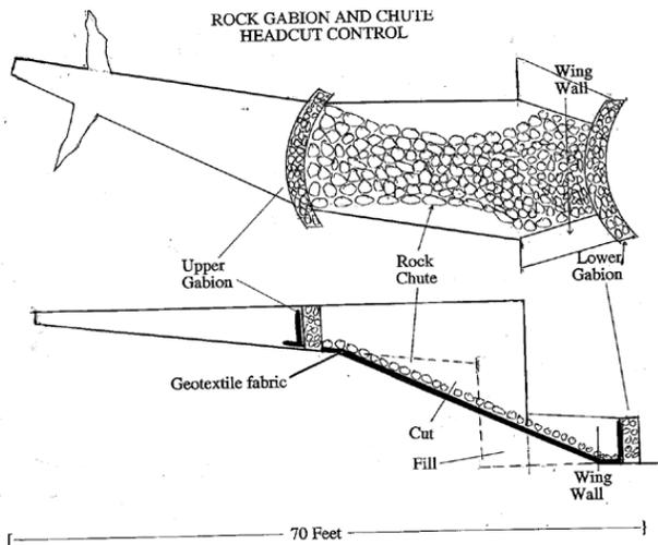
Figure 7. Example 1 control design showing upper and lower headcuts and structures
