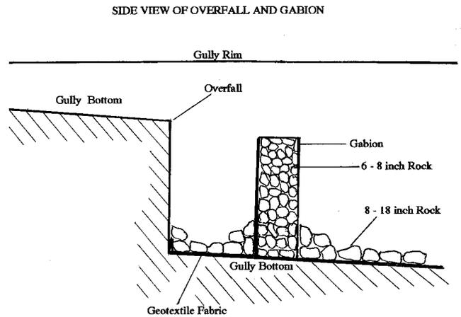
Figure 12. Example 2 control design
