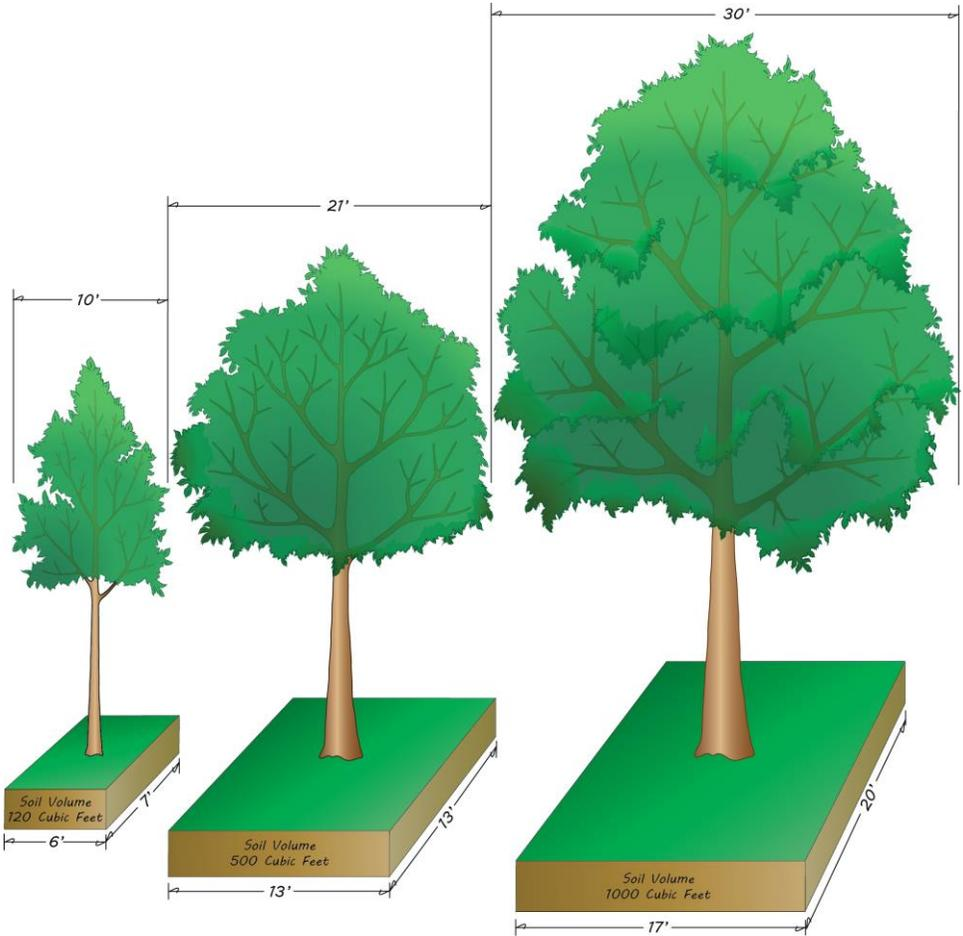
**Figure 3. Tree growth is limited by soil volume. To grow big trees, large amounts of uncompacted soil are needed. For a mature tree with a canopy spread of approximately 30 feet, 1,000 cubic feet of soil is needed. Illustration from Casey Trees, 2008.**
