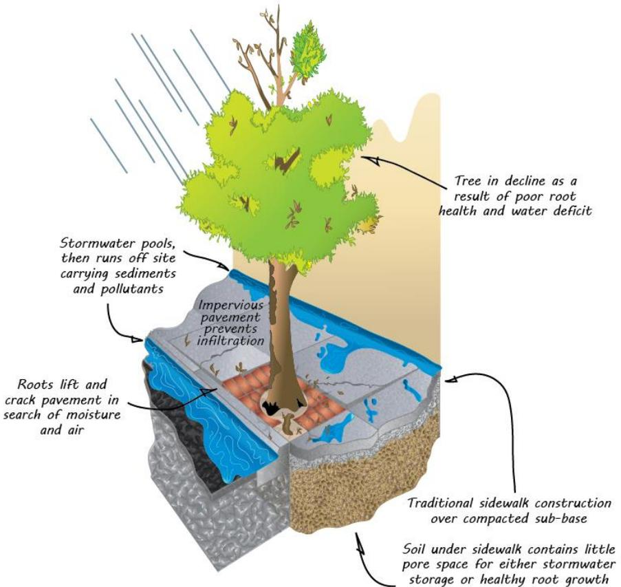
Eventually, and because of poor root health due to site design failures, a tree shows signs of decline and may present an increased risk of limb or tree failure and liability. Often these declining trees are removed because the tree was a problem; however, in reality, it was the site design that was the problem, not the tree. The cost of removing and replacing this tree—a significant investment—is a waste of a community's money and time and it could have been prevented with proper design.
