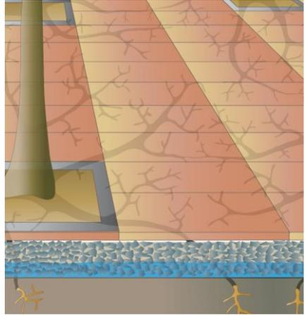
*Permeable pavements (surface shown above) increase infiltration, allowing more runoff to be absorbed and available for use by the tree.*
