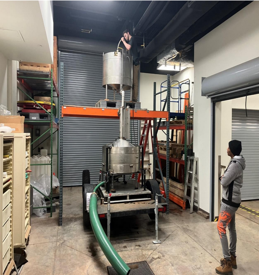
William Krivanek and Termelia Hogg are filling up the 100-gallon prover that was used for the Oklahoma Bureau of Standards' volumetric proficiency test.
