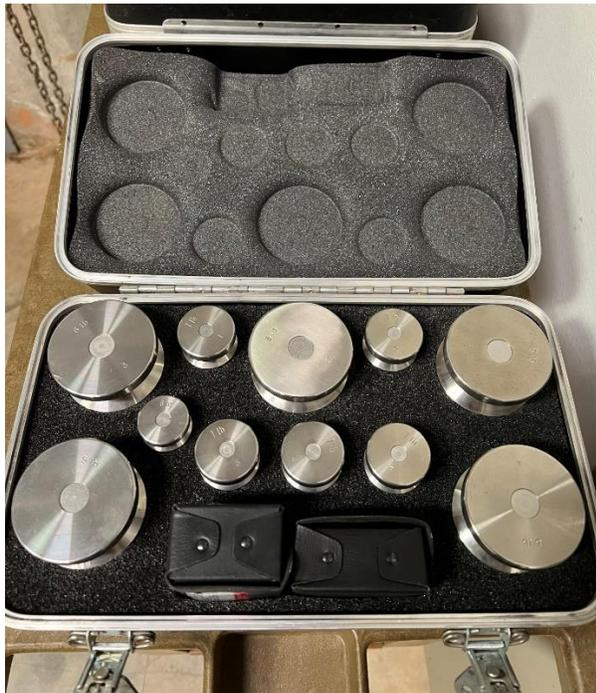
Pictured above: This is a weight kit that was calibrated by the Oklahoma Bureau of Standards during the last week of January. It consists of 31 weights ranging from 5 pounds to 0.001 pounds.
