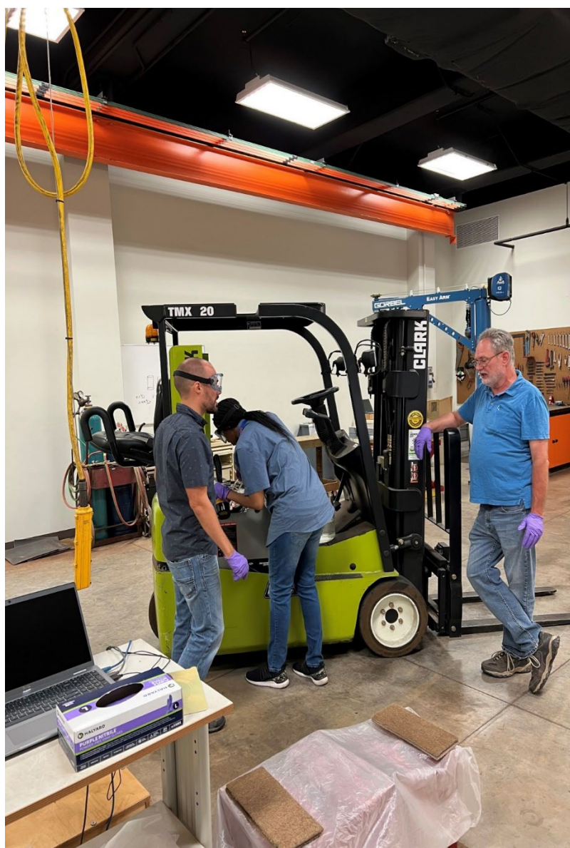
Pictured above: Eli Klimek, Termelia Hogg, and Richard Gonzales are checking water levels on the forklift stationed in the Oklahoma Bureau of Standards.
