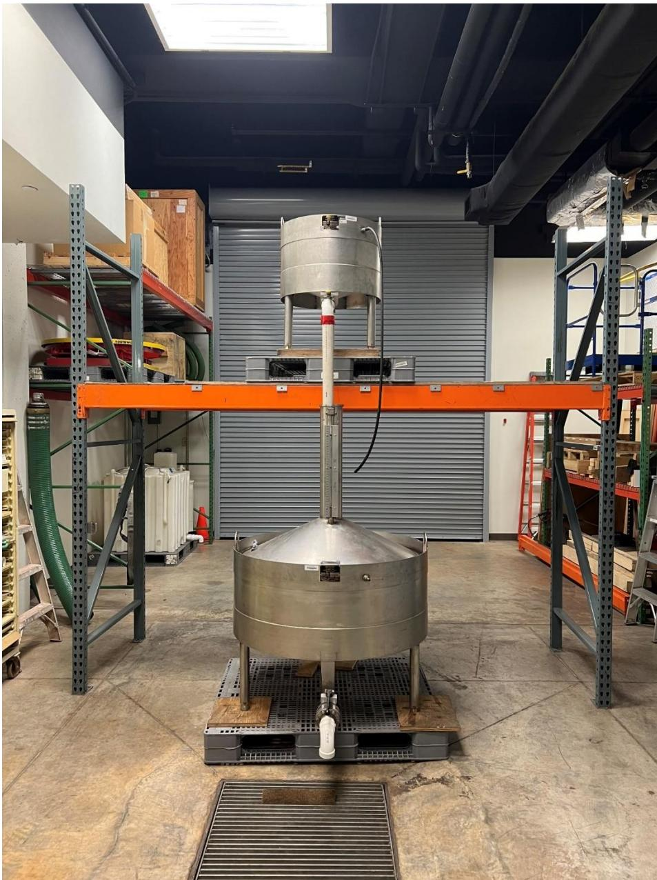
Pictured above: This is the Bureau's scaffold that is used when performing volumetric calibrations on large provers.
