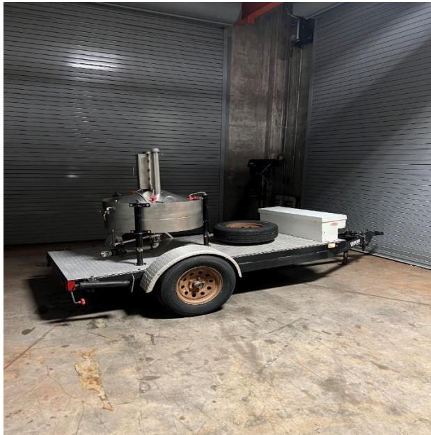
Pictured: This is a 50-gallon volumetric prover that the Bureau calibrates annually for OCC.
