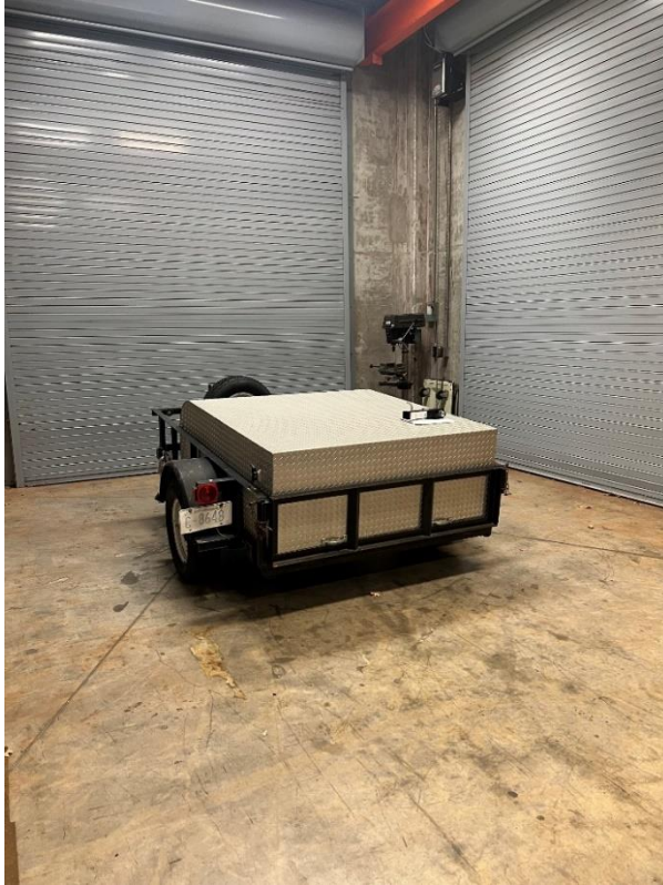
Pictured: This is the trailer that is used to store and transport the 500-pound PT to each state.
