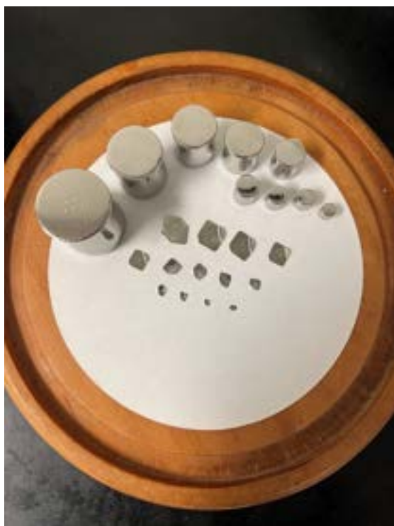
Pictured above: This is a set of standards (100 grams to 1 milligram) from the Mass Echelon II standards pictured above.
