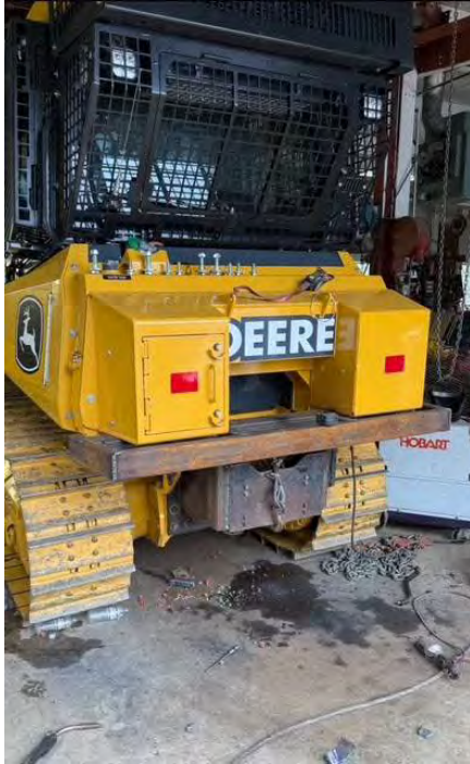
Winch retrofit/Bumper build
