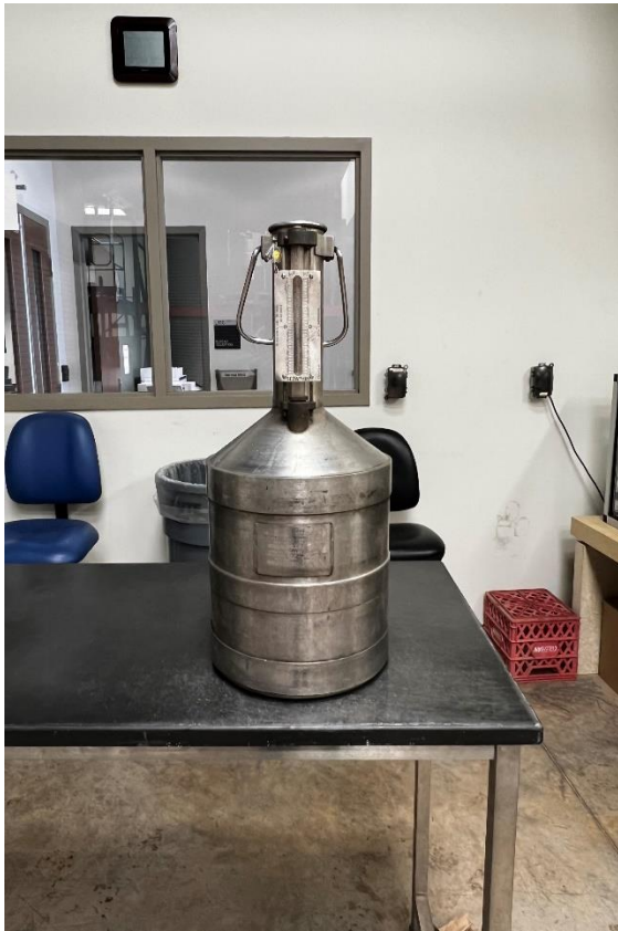
Pictured above: This is a 5-gallon test measure that the Bureau calibrated for a customer.
