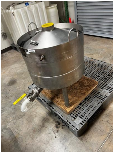
Pictured above is the Bureau's 25-gallon volume standard that was sent to Minnesota for calibration.
